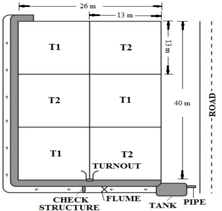
Figure 1. Layout of experimental site
