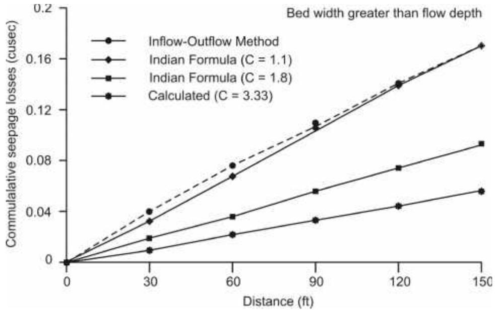
Figure 1. Comparison between Indian Formula and Inflow-Outflow method when bed-width is greater than flow depth.
