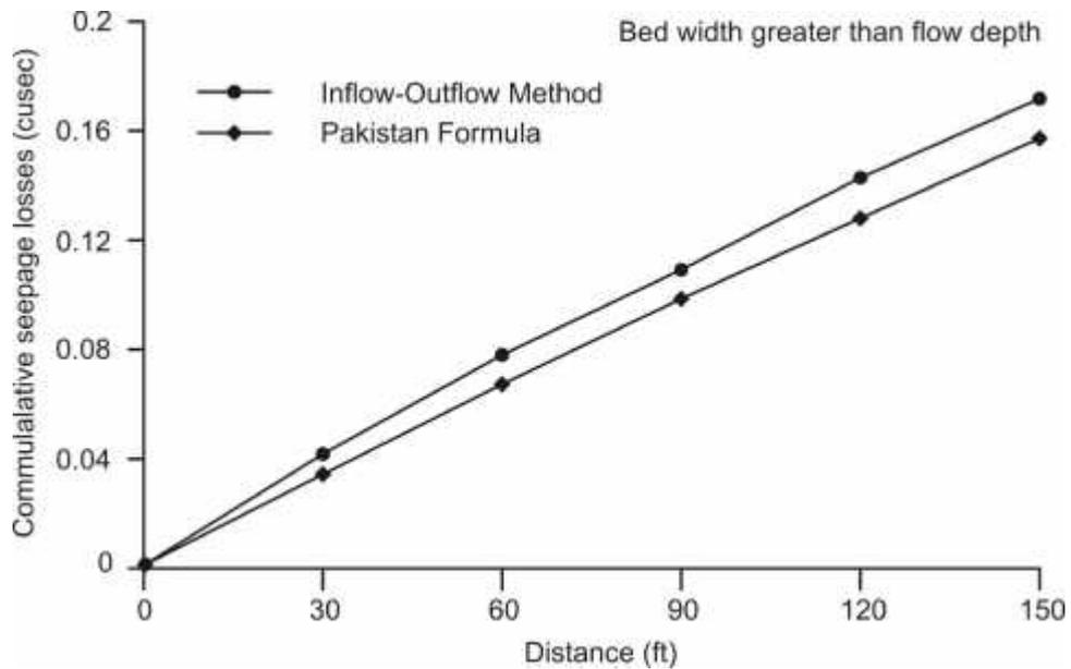
Figure 3. Comparison between seepage measured by Inflow-Outflow method and estimated using formula developed for unlined canals in Pakistan for  $b > d$ .
