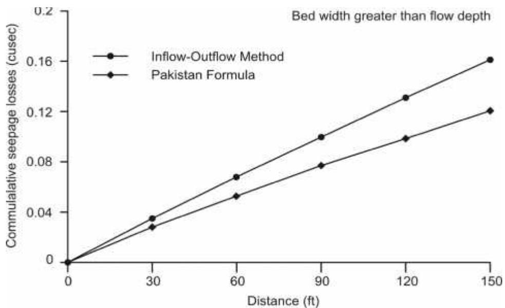
Figure 4. Comparison between seepage measured by Inflow-Outflow Method and estimated using formula developed for unlined canals in Pakistan for  $b = d$ .
