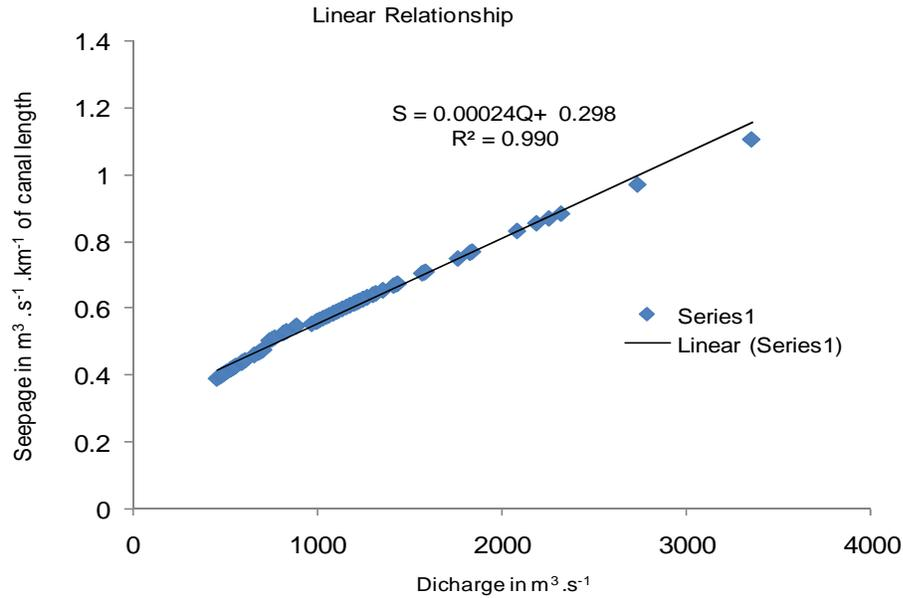
Figure 2. Relationship between seepage and discharge using linear solution.
