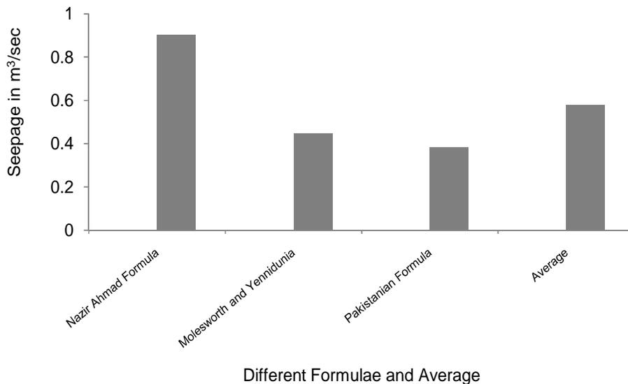
Figure 1. Seepage losses estimated using different formulae
