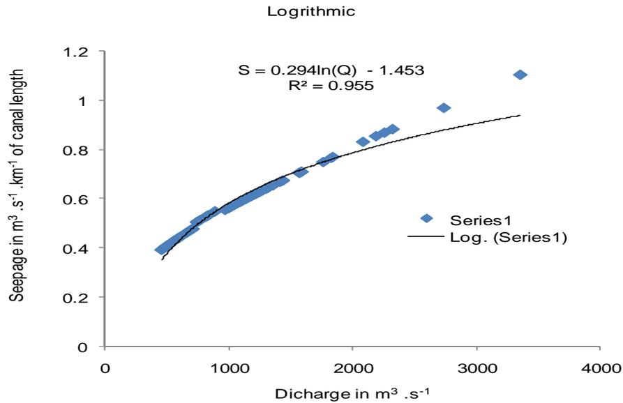
Figure 3. Relationship between seepage and discharge using logarithmic solution.
