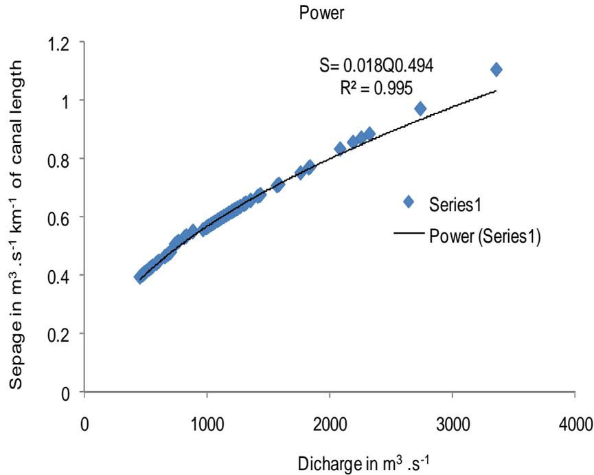
Figure 4. Relationship between seepage and discharge using power solution.
