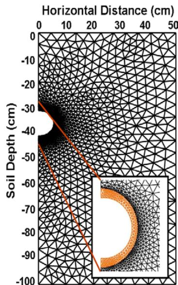
Figure 2. Typical geometry and finite element mesh used in the HYDRUS-2D simulations
