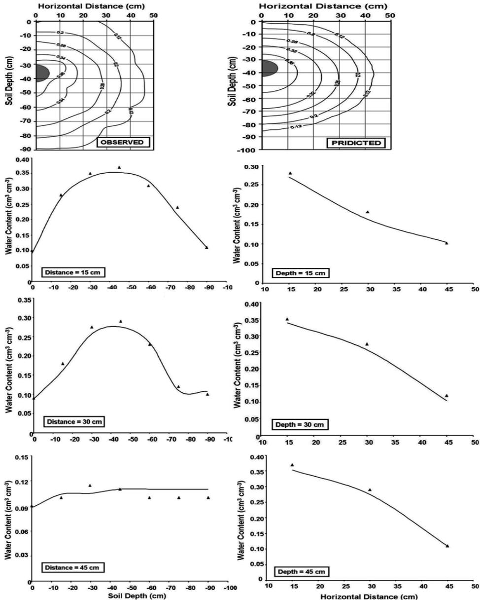
Figure 3. Measured and predicted water contents after five days of irrigation with a constant pipe pressure head of 100 cm.
