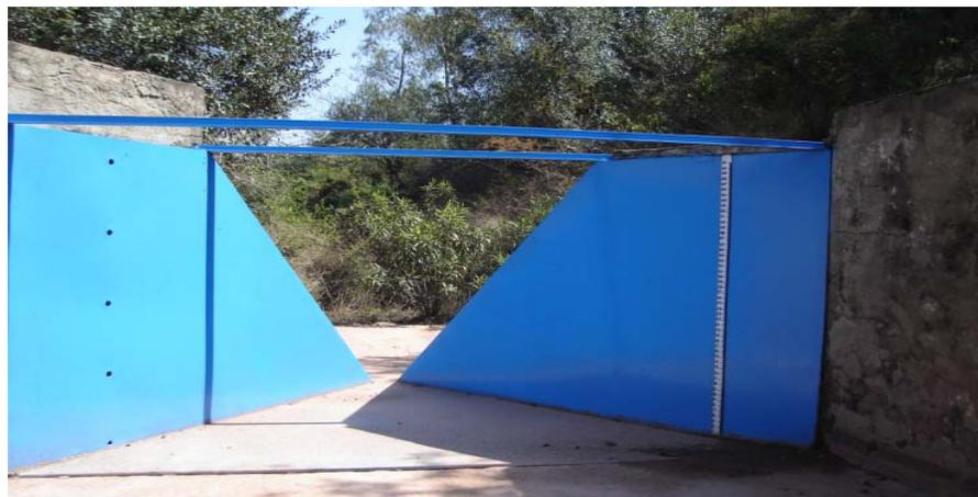
Figure 2. H-flume installed at sub-rawal watershed satrameel
