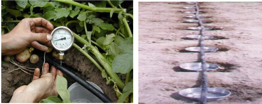
Figure2. Water pressure and emitter discharge along a lateral line
